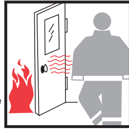
Radiant heat from hot surfaces and flames can cause burns
