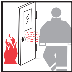
FIG. 6 Radiant heat from hot surfaces and flames can cause burns.
