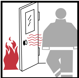
Radiant heat from hot surfaces can cause burns
