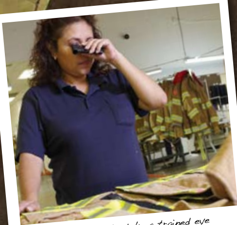
High tech materials take a trained eye to detect performance-threatening conditions. Early detection helps prevent ongoing degradation.
